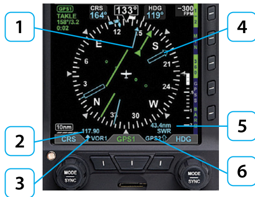
Figure 4-74 Bearing Pointer Description
