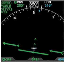
Figure 4-46 Reduced Length Course Pointer, ARC HSI Compass Mode
