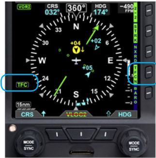
Figure 4-100 Traffic Overlay Enabled
