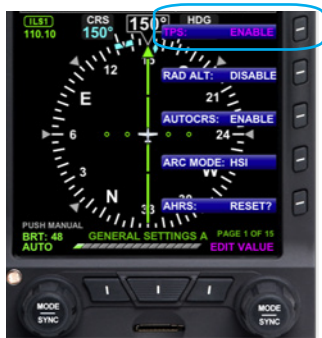
Figure 4-16 Editing Airspeed Tape Display
