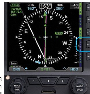
Figure 4-108 GPSS Disabled and Autopilot in HDG Mode
