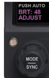
Figure 2-18 Display Brightness in BRT ADJUST Mode
