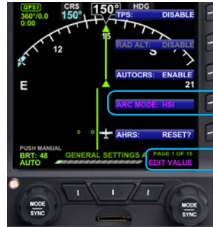
Figure 4-43 Changing the ARC Compass MODE
