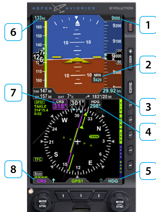
Figure 2-3 Left and Right Knobs and Corresponding Fields
