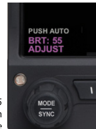
Figure 3-5 Display Brightness in ADJUST Mode
