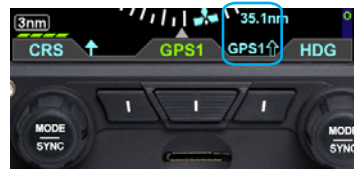
Figure 4-79 Double-Line Bearing Pointer and Button
