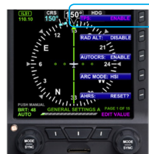
Figure 4-33 Editing Airspeed and Altitude Tape Display
