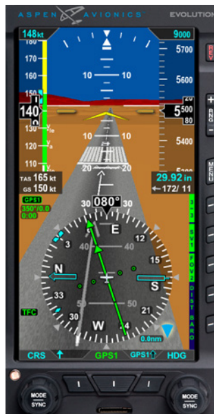
Figure 4-122 Hard-surfaced Runway Display
