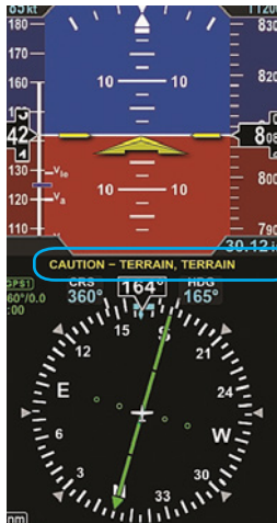
Figure 4-147 Terrain Alert, Synthetic Vision Not Selected
