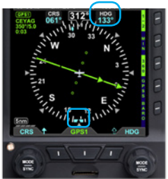
Figure 2-5 HDG field updated and inactive
