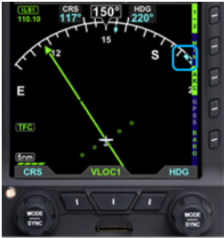
Figure 4-82 Selected Heading Bug Outside of the ARC Compass Scale Range
