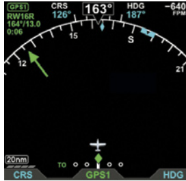
Figure 4-47 Stub Course Arrowhead, ARC CDI Compass Mode
