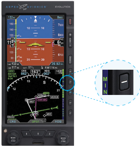
Figure 4-27 MIN Hot Key – Selected MINIMUMS Annunciation and Markers Disabled
