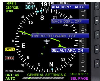
Figure 4-116 Angle of Attack Mode Settings Display
