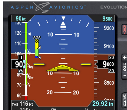
Figure 4-113 Angle of Attack (AOA) Display
