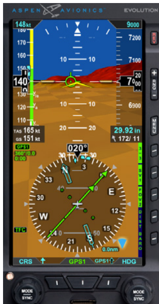
Figure 4-139 Terrain Warning System VIEW
