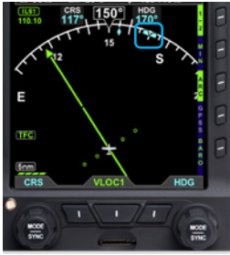
Figure 4-81 Heading Bug and Selected Heading Field
