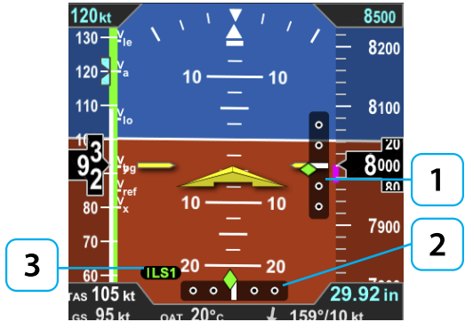
Figure 4-6 Lateral and Vertical Deviation Indicators and Source Information
