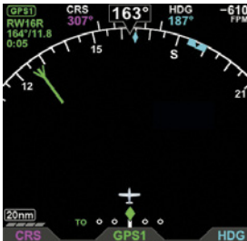
Figure 4-48 Stub Course Tail, ARC CDI Compass Mode
