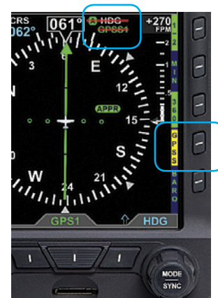
Figure 4-109 GPSS Automatically Disabled — Wings Level Mode
