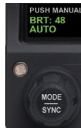
Figure 2-17 Display Brightness in BRT AUTO Mode
