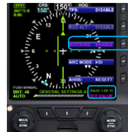
Figure 4-68 AUTO CRS Enabled
