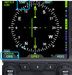
Figure 4-73 CRS Field Enabled for Editing
