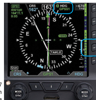
Figure 4-107 GPSS Enabled with Autopilot in HDG Mode
