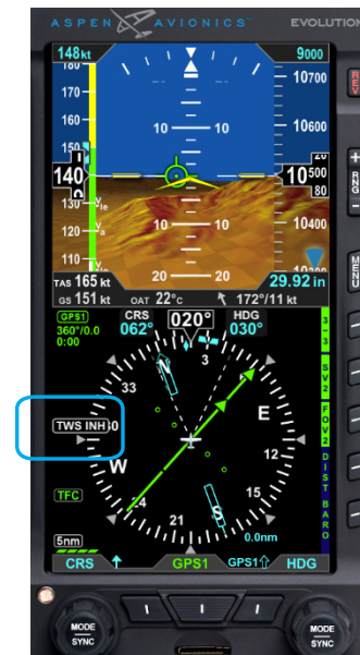
Figure 4-149 TWS Inhibit Display
