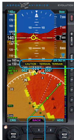
Figure 4-148 Terrain Alert, Synthetic Vision VIEW
