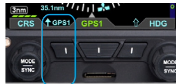
Figure 4-78 Single-Line Bearing Pointer and Button
