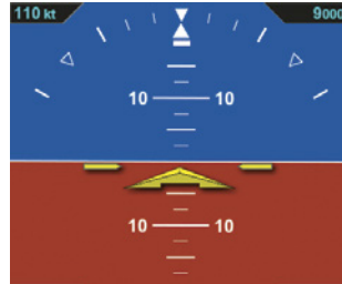
Figure 4-17 Airspeed Tape Disabled
